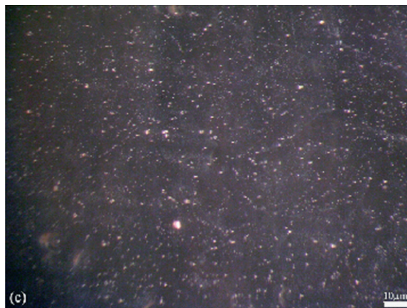
Fig. 1. Nanoemulsion based on Solbrax and ULTRAL L70, which remained stable for over 120 days: (a) photograph (b) droplet size distribution curve and (c) optical micrograph.
